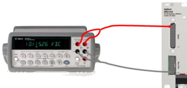
Figure 3-7 Connect the multimeter to the M9216A front panel
