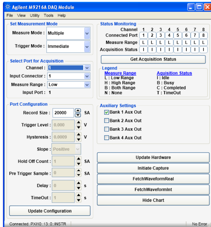
Figure 3-6 Switch Bank 1 Ports to Auxiliary Output
